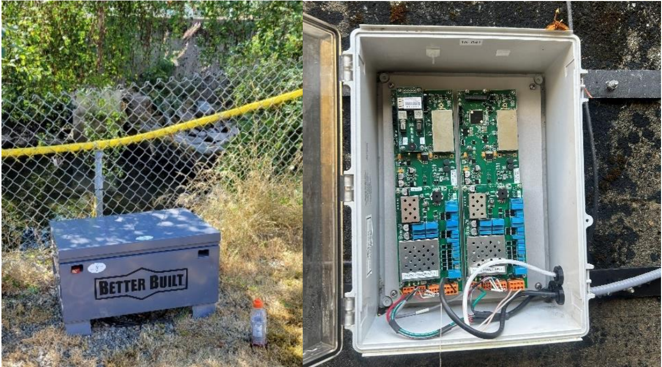
Figure 5. PIT antenna IS1001 reader board housings for Stamp Falls array (left) and the Robertson Creek array (right).
