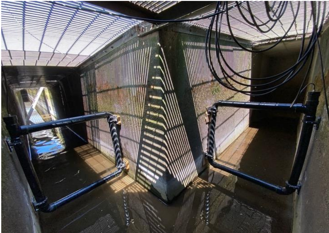
Figure A10. Quinsam River hatchery fishway PIT antennas, 2021 (photo by Jamieson Atkinson).
