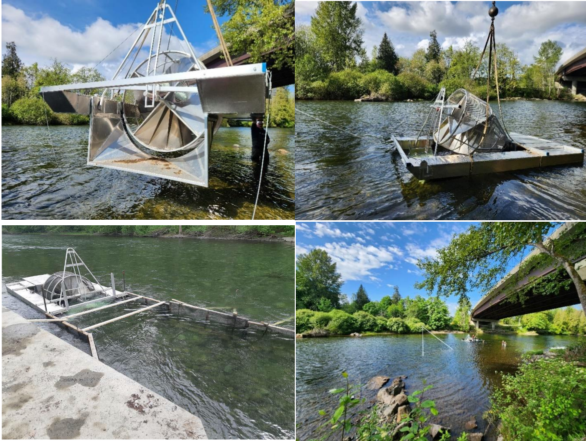
Figure A4. RST-style smolt traps. The upper left image shows the “yolk”, the top left image shows an RST trap not in ‘fishing’ mode. The bottom two images show the different operating methods for RSTs installed in the Cowichan and Nanaimo rivers.
