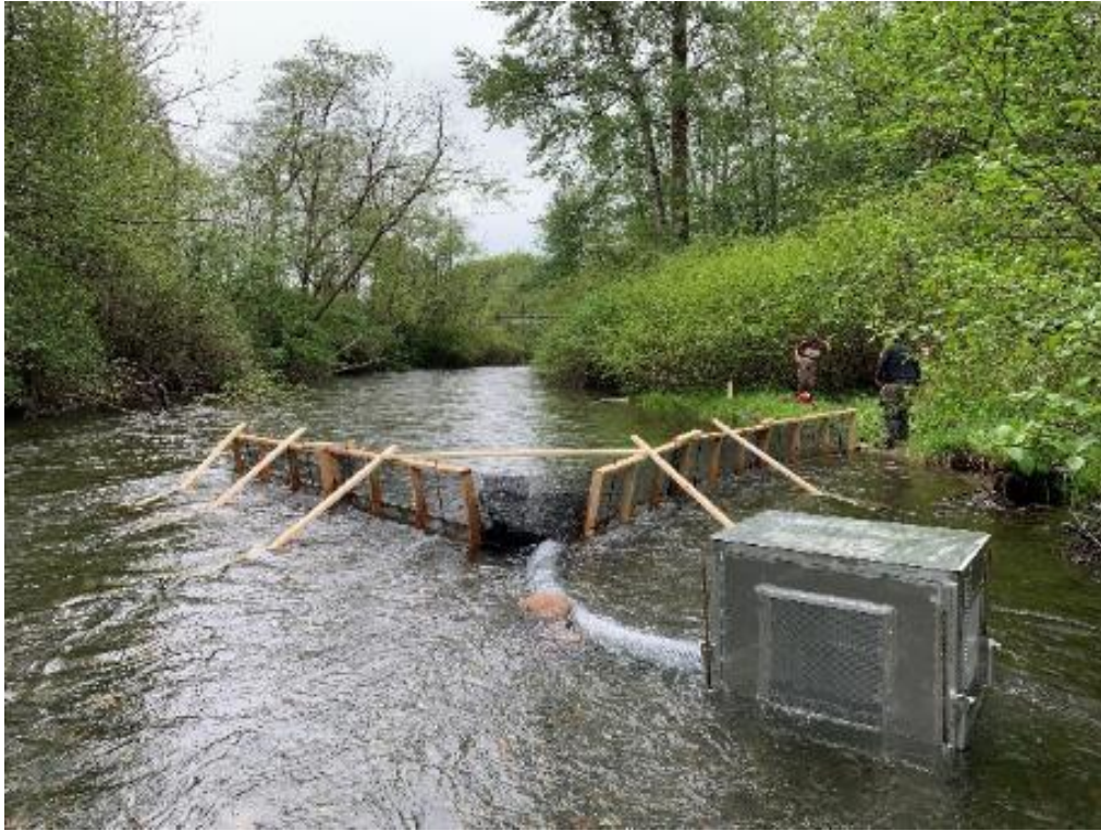
Figure A5. Fence funnelling smolts downstream into a smolt trap.
