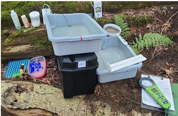
Figure 3. The left image PIT-tagging kit shows the HPR scanner, MK25 tagging gun, pre-loaded FDX-B tagging tray and static baths with MS222 and aerators. The right image shows the 12 mm FDX-B PIT tag.
