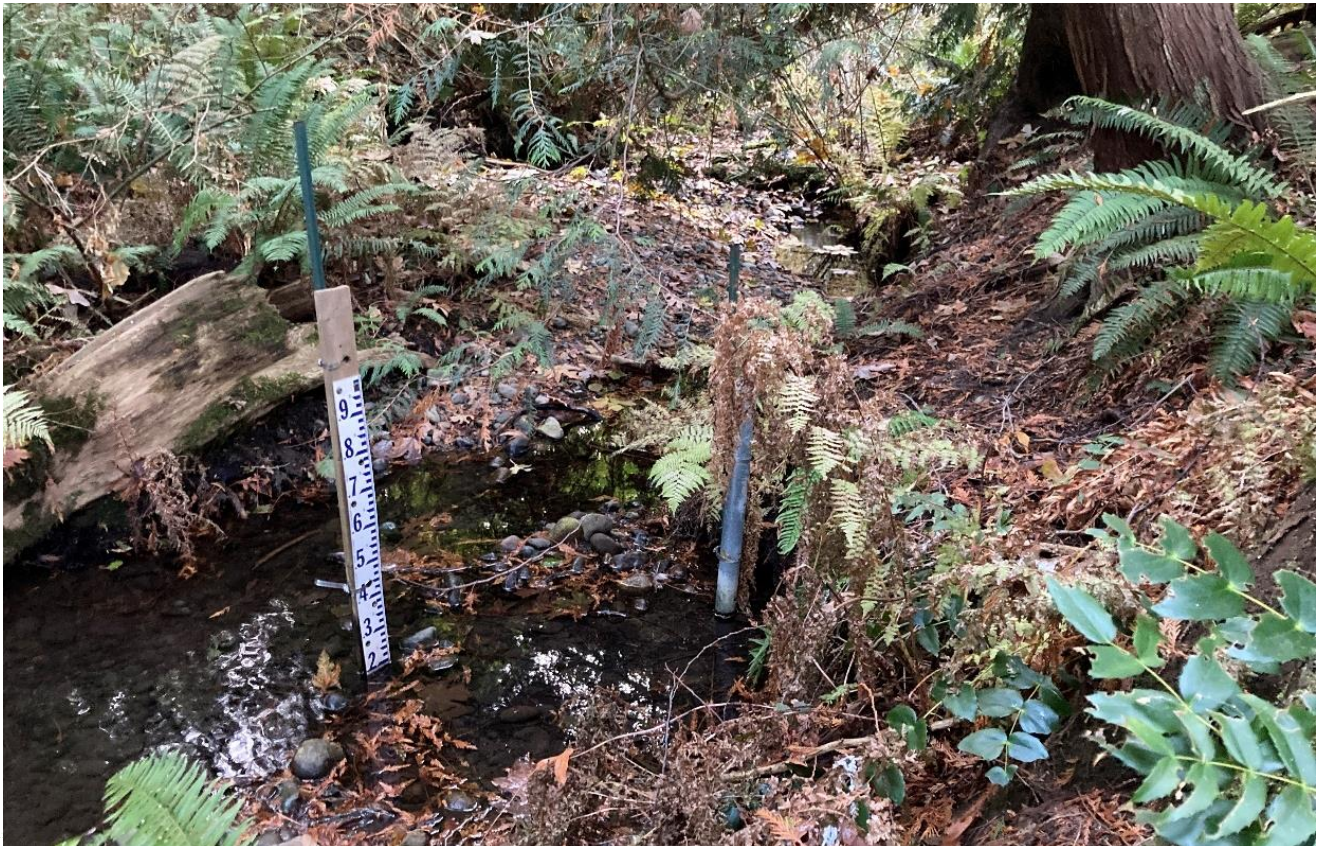
Figure 2. Photo depicts level logger and staff gauge location in Shelly Creek. 2022.
